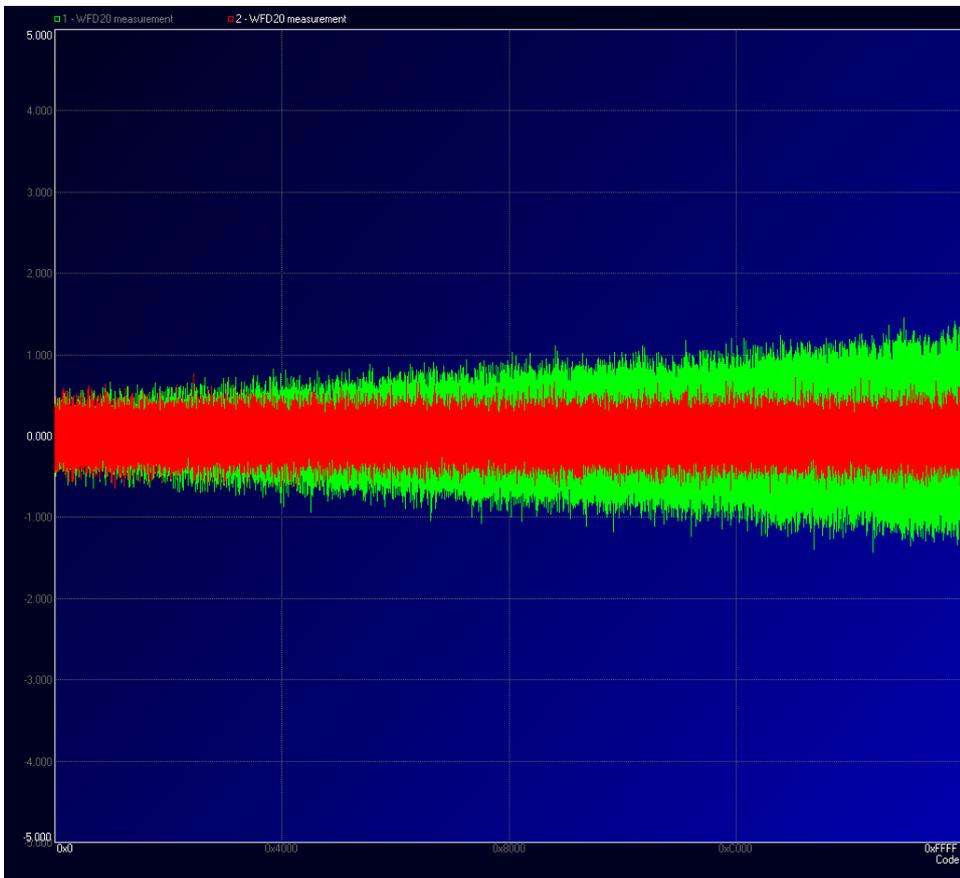
The green plot shows the same converter but now with a 2 wire connection between the ATX reference and the converter. For this measurement, the 500 ohms sense resistor is removed in the test setup. The DNL degradation is also a result of reference GND noise that is normally compensated by the reference GND sense connection.
