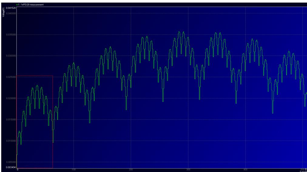
As expected, the enlarged subsection, visualizing the reference current for code 0...512, is divided into eight subsections that are selected by converter bit 6, 7 and 8. Finally, when we zoom in on the first sub section of this figure, we see the change in current when the lowest 6 significant bits are toggled.
