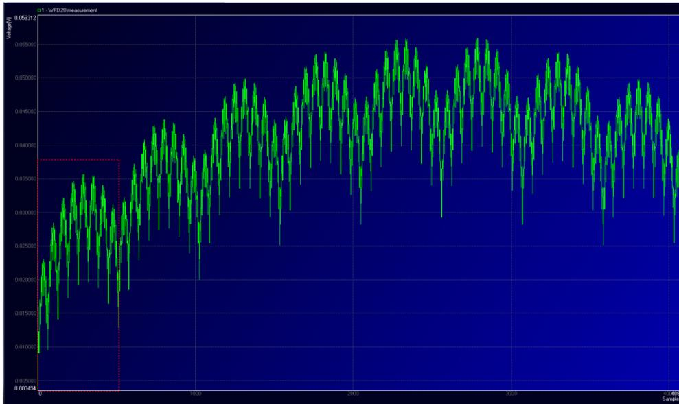
Again, it is clear that this section, on its turn, is again divided in 8 subsections, selected by converter bit 9, 10 and 11. The first sub frame, indicated with the red dotted area, is in its turn enlarged.
