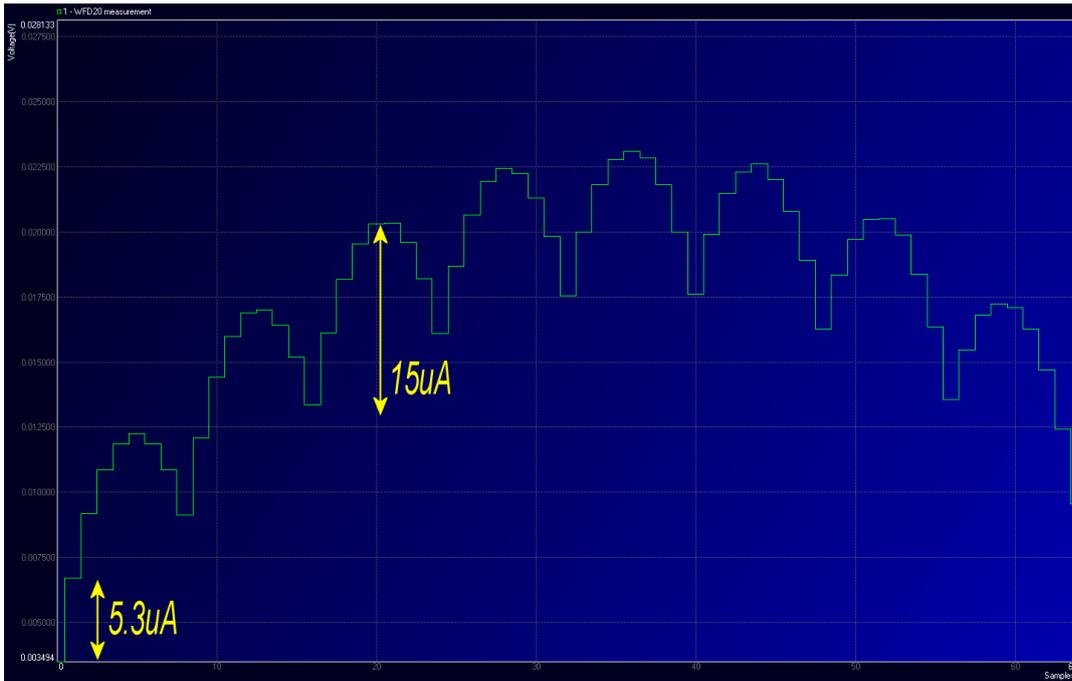
The change in reference current for each code change is clearly unfolded in this graph, for input code 0 to 63.
