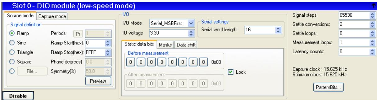
The DIO patternbit generator generates the two clocks needed for the serial data transfer: One internal clock, called SerClk for clocking the DIO shift register. The other one is “User 0” that is used as serial clock for the device under test.
