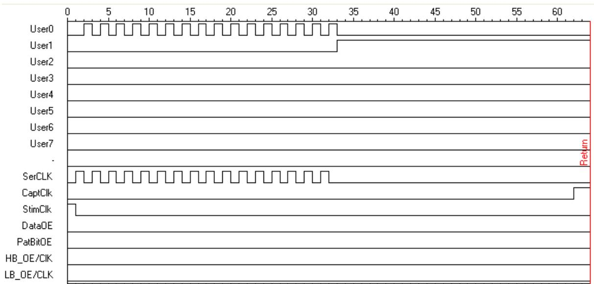
“User1” is connected to the chip select pin of the DUT. After shifting in the Data, the rising edge of CS clocks the serial data into the DAC register.
