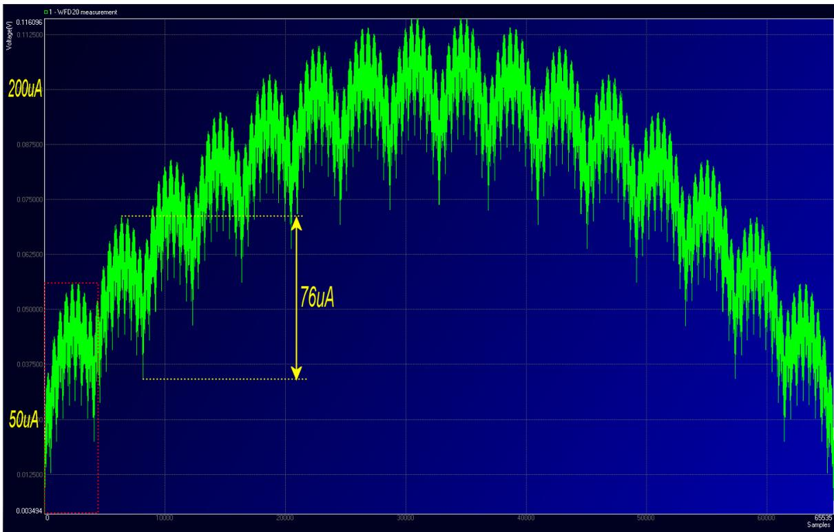
The figure shows a screenshot of the analyzer software, showing the measured voltage over the sense resistor for each converted code. On the horizontal axis are the ADC-codes.
