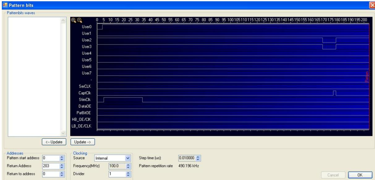
First, Convst is held low for 40ns. Then, after 165 steps (1.65us), the chip select and read lines are taken low to read out the converter result. The capture clock (CaptClk) stores the data into the capture memory. The positive edge of Stimclk, right after Convst, updates the AWG20 module.
