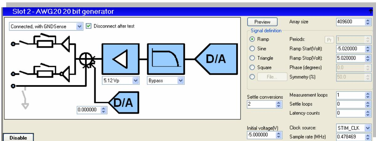
In connection with the high ramp resolution, additional averages are not needed. When needed, the number of measurement loops, or the number of ramp steps may be increased.
