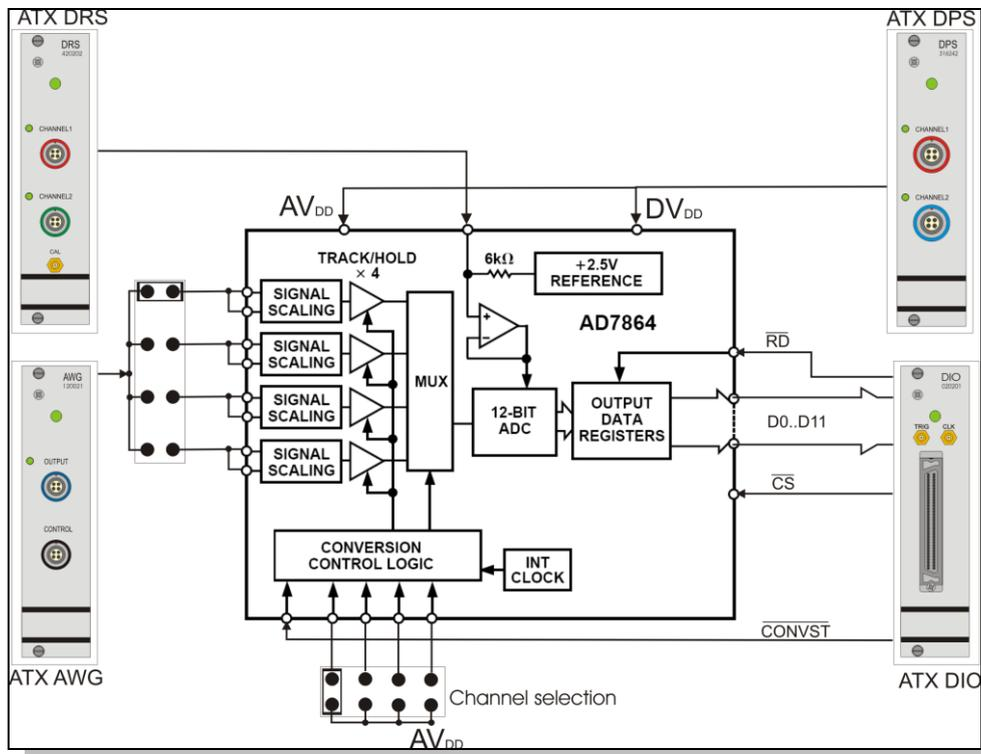
The channel under test is selected by means of two jumpers. The software channel selection option of the device is therefore not used. The input voltage is generated by the ATX7006 AWG20 module. The reference can be connected to the ATX reference module. The device is powered using one channel of the ATX7006 dual power supply module.
