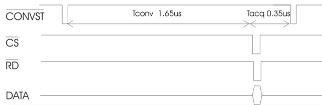
During the acquisition time the sample and hold is acquiring the analog input. The output of the AWG20 module is settled a considerable time when it is sampled right after a conversion start.
